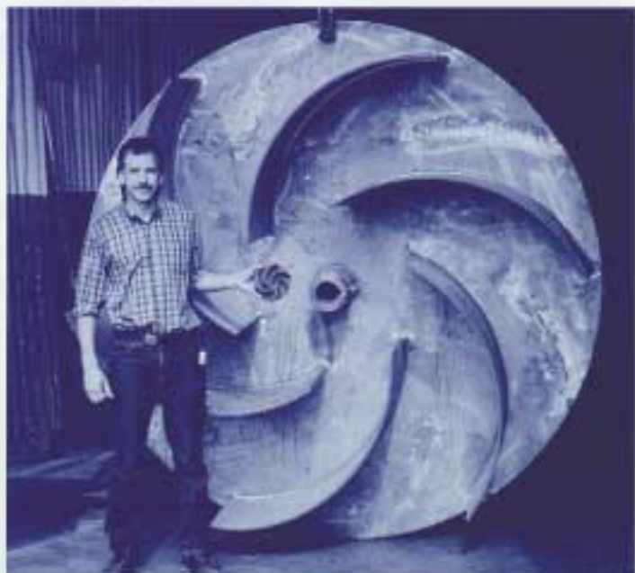
Senior Research Technician Dick Howk shows lab-size impeller compared to full-size version.
