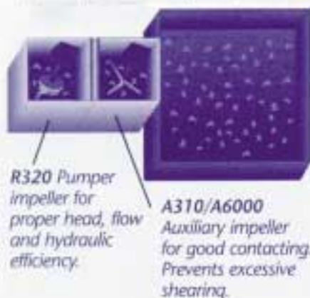
Figure 2. First Stage Extractor Transfers most of the Cu from the aqueous phase to the organic phase.
