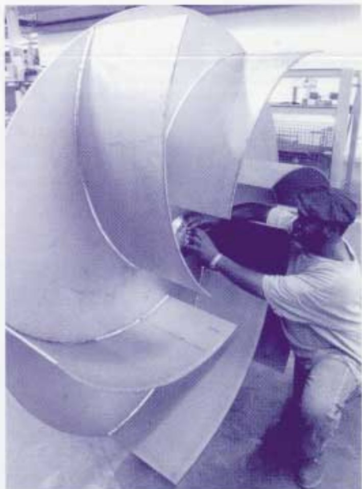
Jim Simmons checks the hub alignment and fit of an R320 impeller before shipment.
